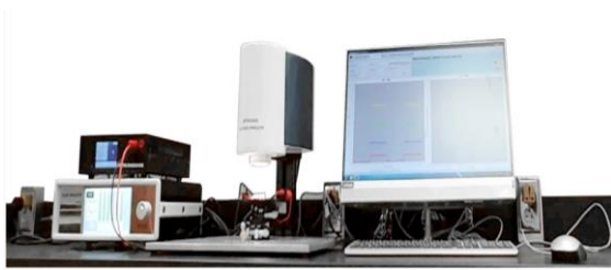
Fig. 2. FYTRONIX 8000 Solar IV and CV characterization system
