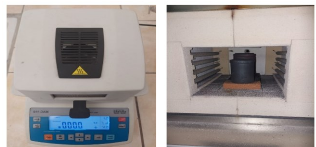
Figure 3. a) Moisture Device b) Muffle Furnace
