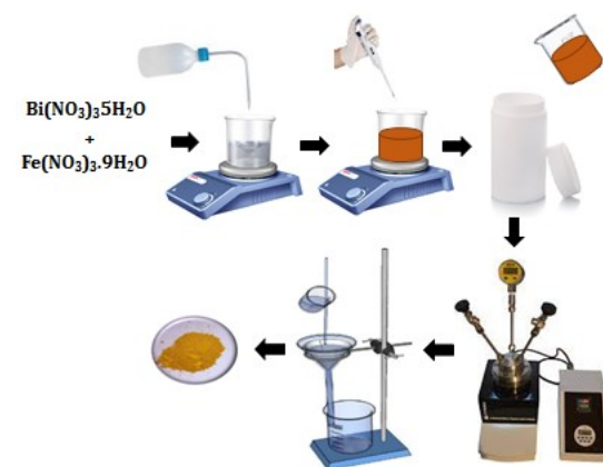
Fig.1. Schematic representation of the hydrothermal method process
