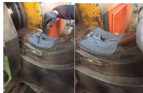
Fig.2. Visual demonstration of connecting the mold to the extruder.
