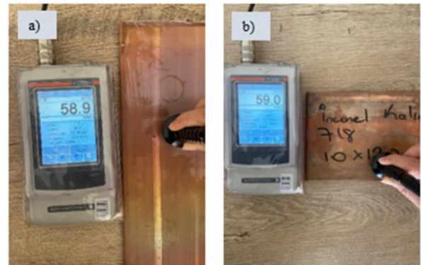
Fig.6. a) X38CrMoV5-3 (1.2367) and b) Inconel 718 extrusion die; display of conductivity measurements of final products.
