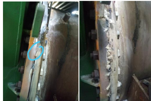
Figure 7: Seal and welding applications in the flange regions of the valves
