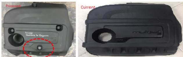
Fig.6: Photographs of Proposed and Current Engine Covers after Dimensional Stability Test, Thermal Cycling Test, Extended Heat aging Test and Heat Shock Test
