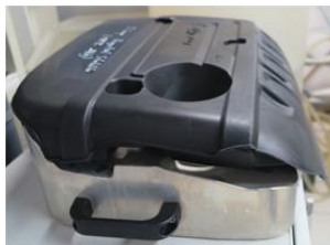
Fig.5: Engine Cover Fixture Simulating the on-Vehicle Conditions
