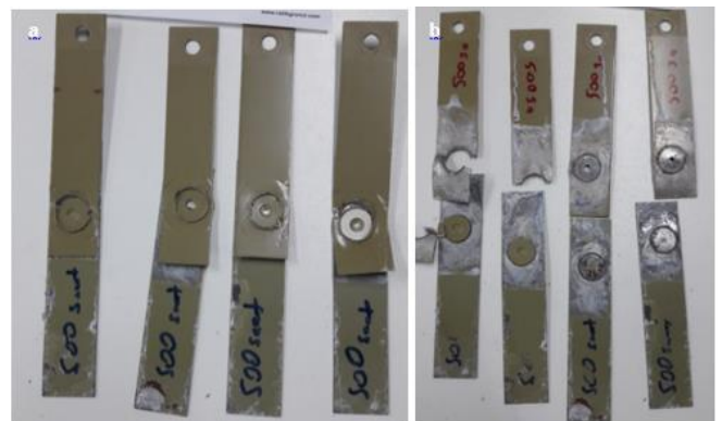
Figure 16. Samples with e- coat application after 500 hours a) after the samples have been subjected to tensile test b) same samples separated from the joint area in order to observe the weld zones
