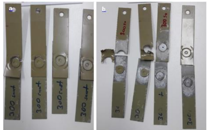
Figure 15. Samples with e- coat application after 300 hours a) after the samples have been subjected to tensile test b) same samples separated from the joint area in order to observe the weld zones
