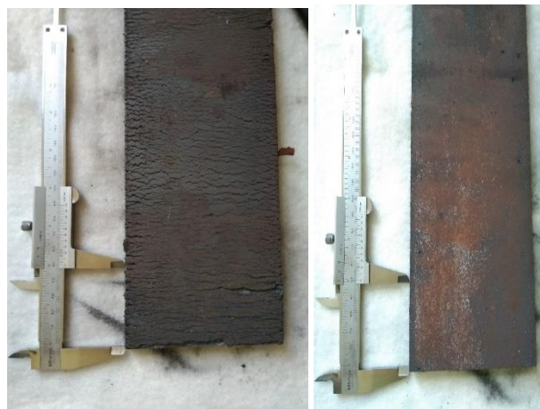
Figure 1. Determination of Surface Edge Cracks with Calliper.
